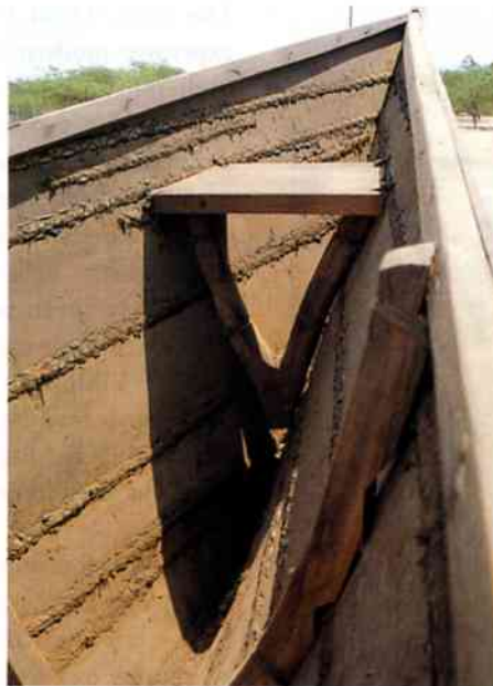
Sewn boat in Oman, a typical example of sewn boats all around the Indian Ocean.
